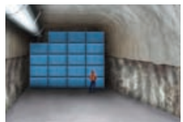
Low level waste emplacement room.
